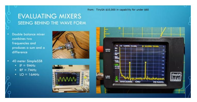
Note that for the double balanced mixer only the sum (16+7=23MHz) and difference (16-7=9MHz) frequencies are present. Neither of the original frequencies (16MHz, 7MHz) show any power in the display.
