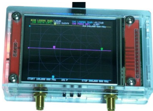
NanoVNA V2 with push buttons (S-A-A-2) by OwOComm V2 Plus V2.3 2.8" display 50 kHz – 3 GHz
